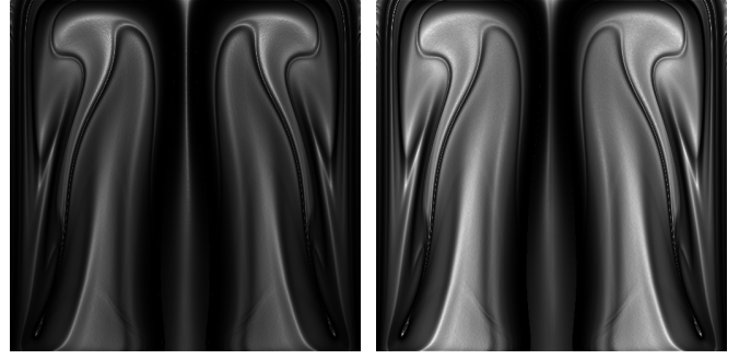
Fig. 5. Comparison of planar FTLE vs. a section of 3D FTLE in the cylinder dataset (dark areas correspond to high values of forward FTLE). The chosen section is perpendicular to the lid and contains the cylinder axis.
