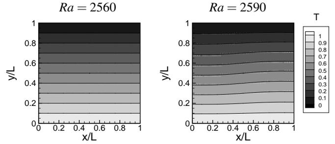
Figure 4. Dimensionless temperature fields corresponding to flows at  $Ra = 2560$  (pure conduction) and  $Ra = 2590$  (weak convection).
