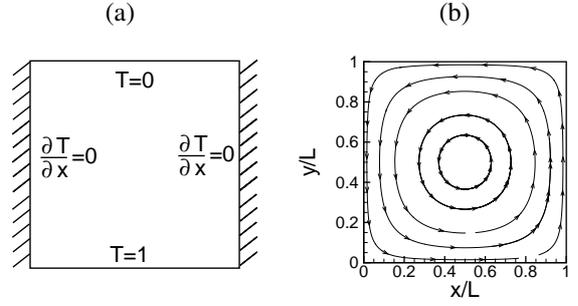
Figure 3. (a) Schematic of the geometry and boundary conditions. (b) Rayleigh-Bénard roll at Rayleigh number  $Ra = 2590$ .
